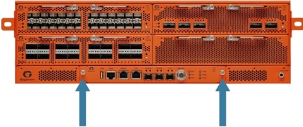
Figure 15 Extension Board Screw Location on GigaVUE-HC3 Front
