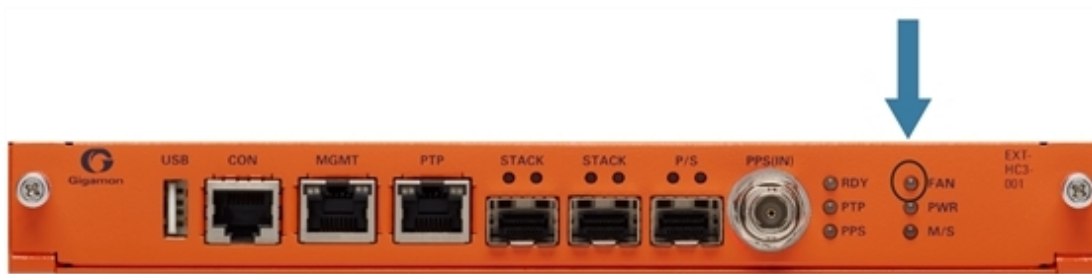
Figure 5 Global Fan LED Location on GigaVUE-HC3 Front
